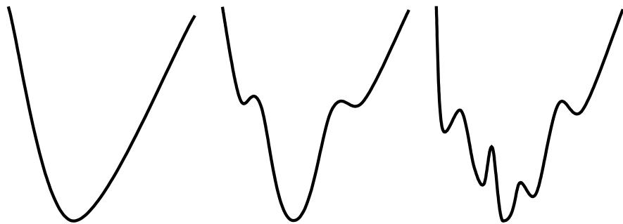
**Figure 7.7:** Principle of Graduated Non Convexity: at first, the energy functional is “convexified”; when the minimum for this energy functional is reached, its convexity is decreased, and the minimum of this functional is computed. This procedure is repeated until a reliability criterion is satisfied.
