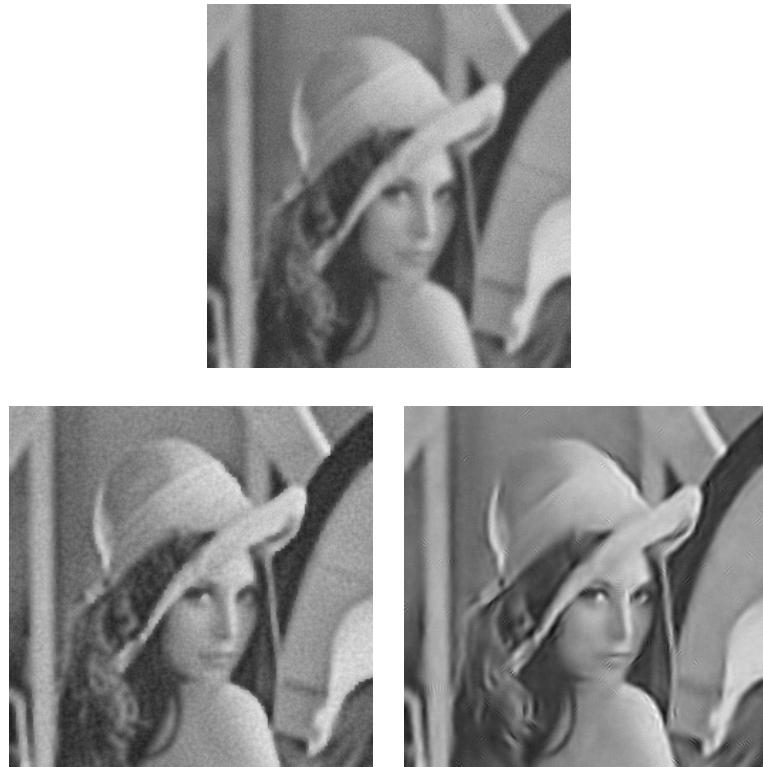
**Figure 7.9:** A preliminary result of our GNC-based method. Top: the degraded image. Bottom left: result of the spatial version of the GNC-based method (with constant  $\lambda$  and  $\mu$ ). Bottom right: result of our multiscale GNC-based method.
